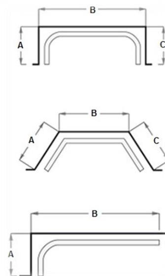
If a corner is not at 90 degrees (EG scenario 2), an "angle finder" is recommended to measure the bend.
