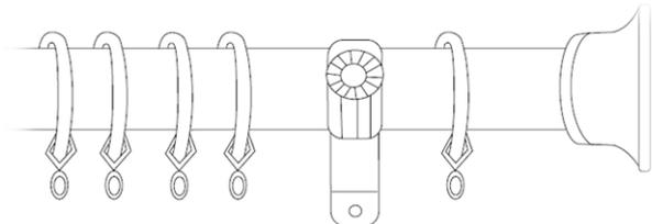
Ring Rod comes maximum 3 brackets as rings or eyelets cannot pass through any brackets.
